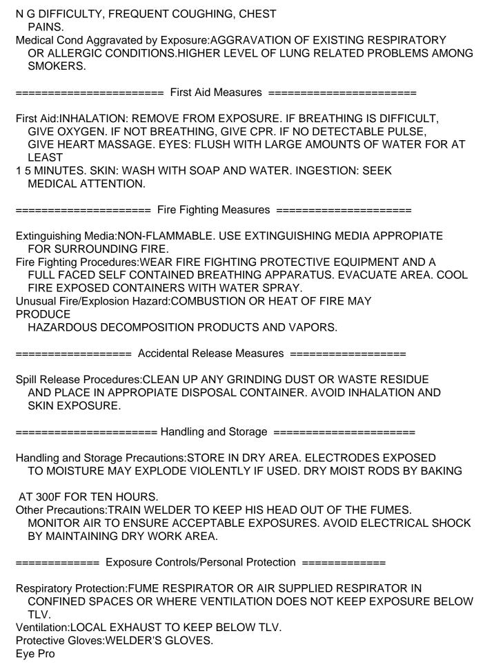
tection:HELMET OR FACE SHIELD WITH FILTER LENS.
